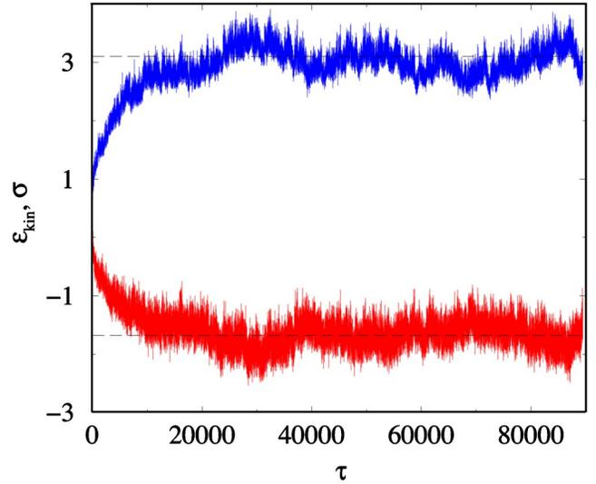
FIG. 7. Time dependence of the kinetic energy  $\epsilon_{kin}$  (top) and the virial variable  $\sigma$  (bottom) of the collapsing uniform state with  $\epsilon = -0.5$  and  $N=125$ . The dashed horizontal lines indicate the equilibrium values of  $\epsilon_{kin}$  and  $\sigma$  of the corresponding core-halo state.
