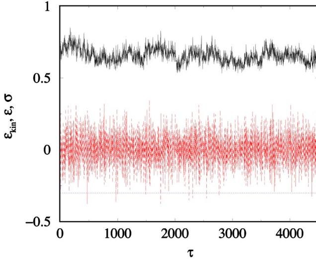
FIG. 3. Plots of time dependence of kinetic energy  $e_{kin}$  (solid line), virial variable  $\sigma$  (dashed line), and total energy  $\epsilon$  (dotted line) for a uniform system of  $N=250$  particles at  $\epsilon=-0.3$ .
